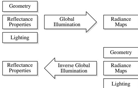
Figure 1: **Overview of the Method** This figure shows the relationship between global illumination and inverse global illumination. Global illumination uses geometry, lighting, and reflectance properties to compute radiance maps (i.e. rendered images), and inverse global illumination uses geometry, lighting, and radiance maps to determine reflectance properties.
