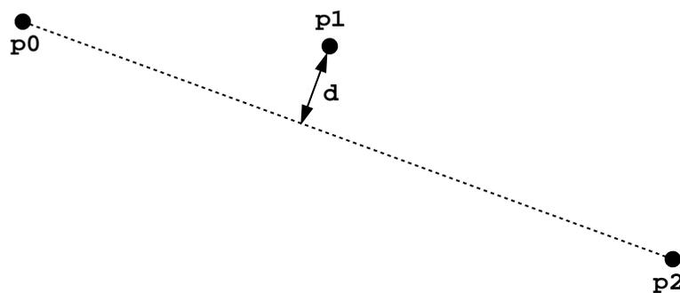
Figure 4.6: The distortion error function for a single line of three world-collinear points. The error is the distance  $d$  between the middle point  $p_1$  from the line connecting the endpoints  $p_0$  and  $p_2$ . This error is summed over many triples of world-collinear points to form an objective function, which is then optimized to determine the radial distortion coefficients of the lens.
