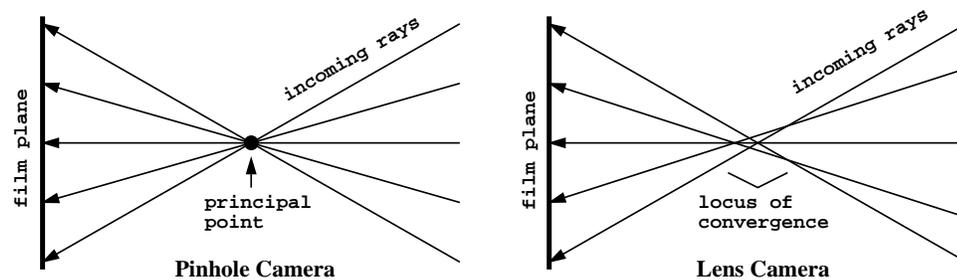
Figure 4.1: In a pinhole camera, all the imaged rays must pass through the pinhole, which effectively becomes the mathematical location of the camera. In a real camera with a real lens, the imaged rays need not all intersect at a point. Although this effect is usually insignificant, to treat it correctly would complicate the problems of camera calibration and 3D reconstruction considerably.
